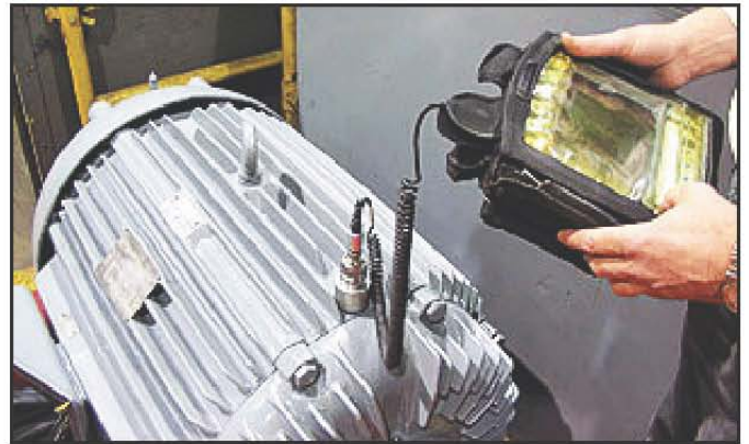
Transducer picks up vibration signals from bearing locations and transmits them to a data collection device.
